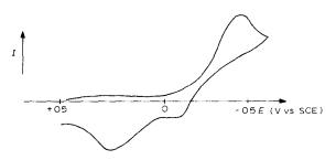
Fig. 1. Cyclic voltammogram of  $[Co(CO)_4]_3$ SnCl in 0.1 *M* TBAP DME solution with a hanging mercury drop cathode. Scan rate 50 mV s<sup>-1</sup>
